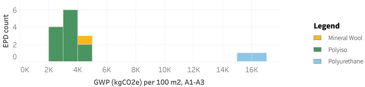
**Figure 4. Product EPD GWP by insulating material.** Some IMP products with a proprietary hybrid foam core are grouped here with polyiso as polyiso is a similar generic insulating material in terms of R-value and GWP.<sup>2</sup> The polyurethane core products have a much higher carbon footprint due to the use of HFC blowing agents that emit to the atmosphere during foam production.
