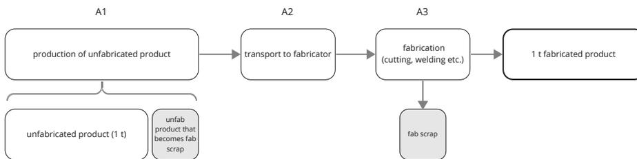
**Figure 2. Life cycle stages and fabrication scrap in fabricated steel product EPDs.**
