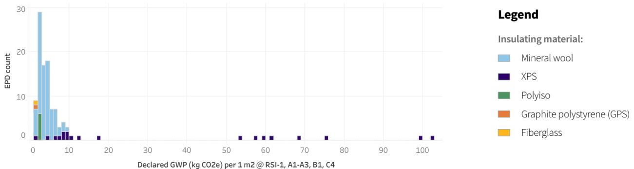
Figure 11. Board insulation product EPDs by insulating material.
