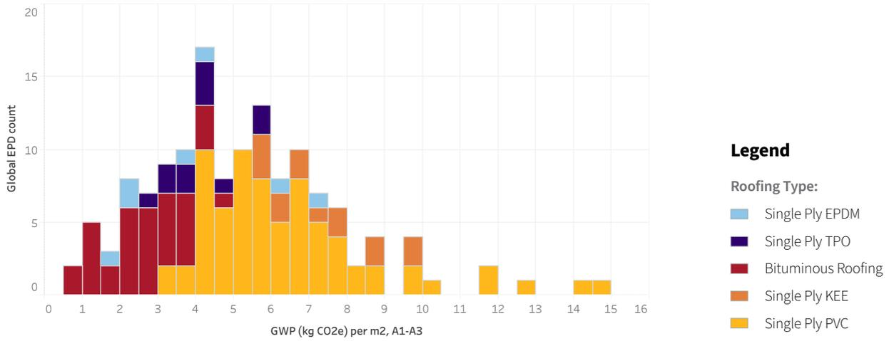
**Figure 7. Global roofing membrane product EPDs by type and GWP.** These EPDs may not be comparable: some use different PCRs and products may not be functionally equivalent (due to different material type, thickness, service life, etc.)
