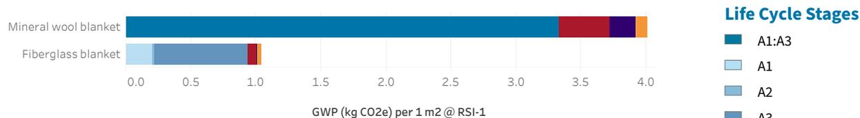
**Figure 1. GWP Contribution by Life Cycle Stage.** The IW-EPD for mineral wool light-density board (considered as “blanket” for this study). There is no IW-EPD for fiberglass blanket insulation. The data included here for fiberglass is from one product EPD and may not be representative of the industry.<sup>4</sup>
