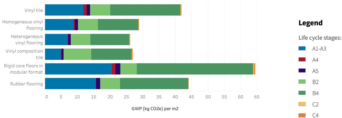
**Figure 1. GWP contribution by life cycle stage, over a 75-year building service life.** A1–A3: raw materials acquisition and manufacturing; A4: transport to site; A5: installation; B2: maintenance; B4: replacement; C2: end-of-life transport (barely visible in chart); C4: disposal.
