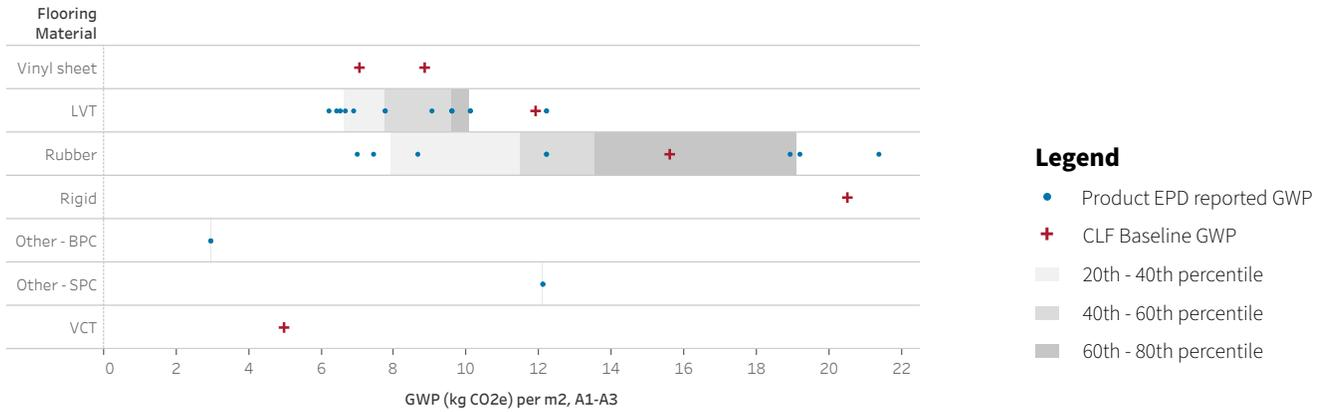
**Figure 2. Range of applicable product EPDs and CLF Baselines.** “Vinyl sheet” includes both homogenous and heterogenous vinyl flooring. “Other - BPC” refers to biobased polyester composition floor tile (2 identical GWP results). “Other - SPC” refers to stone polymer composite (2 identical GWP results).
