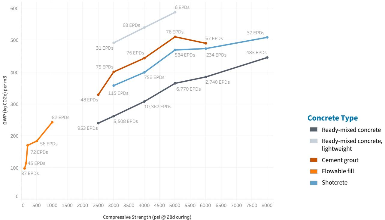
**Figure 1. Concrete GWP and EPD count by type and compressive strength.** This chart describes USA concrete EPDs. Each type-compressive strength data point (e.g., shotcrete-4000 psi) includes a count of the applicable product EPDs in CLF’s data set and the average A1-A3 GWP per m<sup>3</sup> (location along the y-axis).
