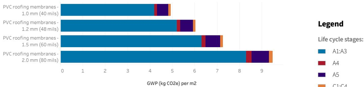
**Figure 1. GWP contribution by life cycle stage.** A1:A3 raw materials acquisition, transport of raw materials, membrane manufacture; A4 transport to building site; A5 installation (mechanically fastened for this IW-EPD); C1:C4 end-of-life: disposal and recycling.
