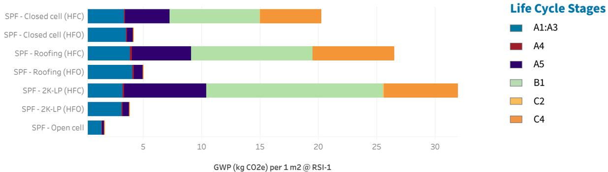
**Figure 2. GWP Contribution by Life Cycle Stage.** The IW-EPDs for spray polyurethane foam insulation aggregate stages A1-A3, and also include stages A4, A5 (when the foam is produced on-site), B1 (accounting for blowing agent emissions during the life of the building), C2 (negligible impacts), and C4 (dominated by blowing agent emissions after disposal).<sup>1,2</sup>
