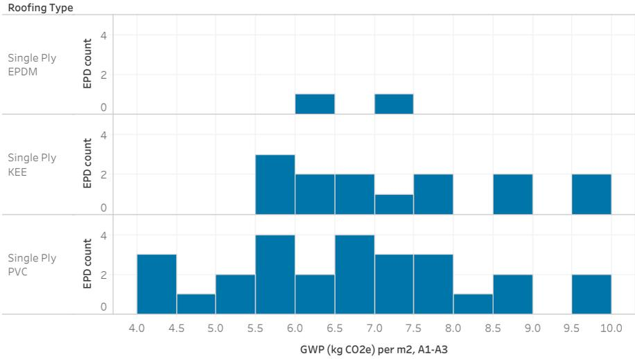
**Figure 3. Distribution of applicable product EPDs.** The chart shows data for products with a range of different thicknesses.
