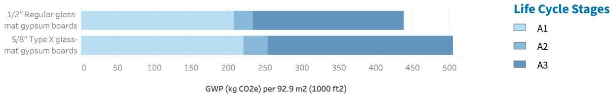
**Figure 1. GWP Contribution by Life Cycle Stage.** A1: extraction and upstream production, including mining to procure gypsum ore and cradle-to-gate glass matting production. A2: transport to factory. A3: glass-mat gypsum board product manufacture. See Section 4.2 System Boundary in the IW-EPD background LCA report for further discussion of all processes and where they are accounted for.<sup>1</sup>
