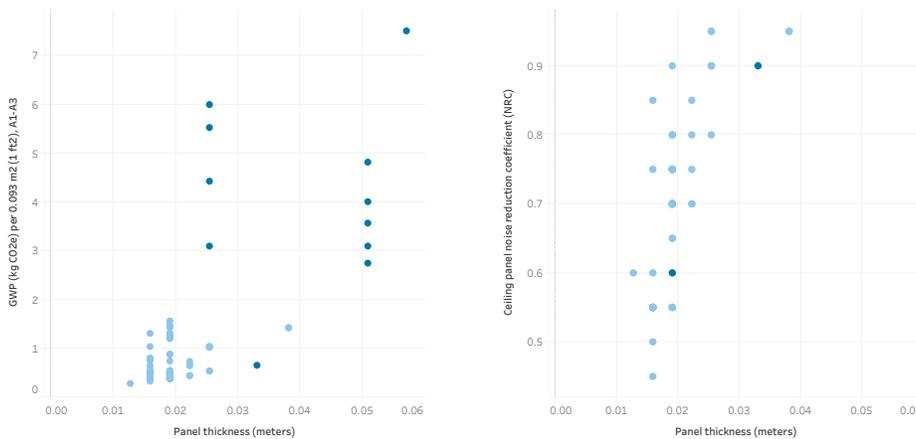
**Figure 5. Relationship between panel thickness and GWP (left) and NRC (right).**
