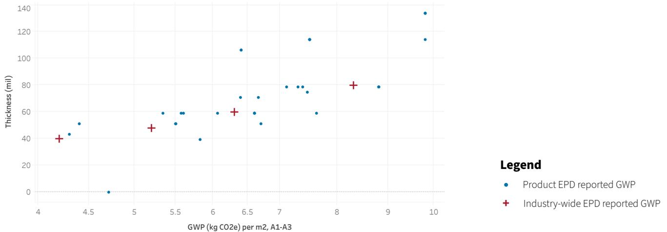
Figure 6. Relationship between roof membrane thickness and GWP.
