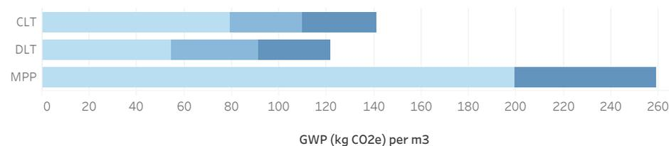
**Figure 1. GWP contribution by life cycle stage.** As there are no industry EPDs for this product type, the information displayed here is from product EPDs. For DLT and MPP, this is based on the one EPD available for each.<sup>4,5</sup> For CLT, this is based on an average of the collection of applicable product EPDs.
