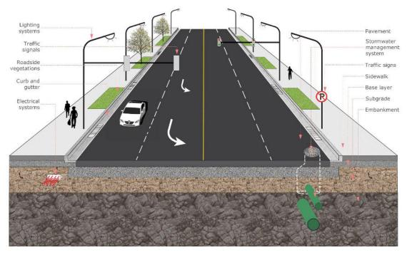
**Figure 1.** Roadway infrastructure components include not just pavement, but also sidewalks, traffic signals, lighting systems, stormwater management systems, curbs and gutters, sanitary water conveying systems, embankments, among others. *Graphic Credit: Sindhu Raju.* © *Carbon Leadership Forum*
