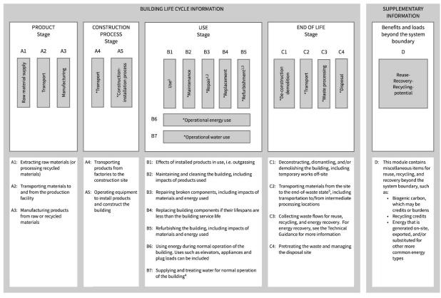
Figure 3.1. LCA stages and modules per EN 15978, reproduced from Life Cycle Assessment of Buildings: A Practice Guide.3
