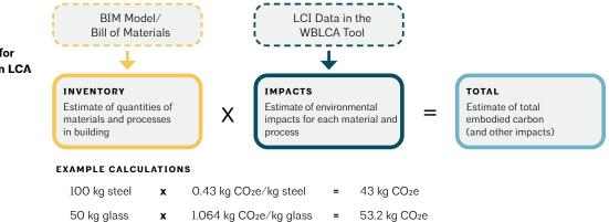
FIGURE 2 Calculation process for impact assessment in LCA
