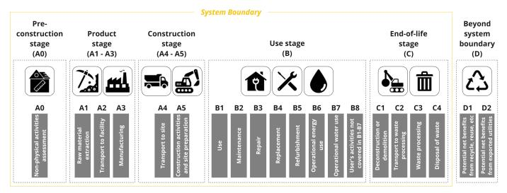
Figure 1. Life cycle stages and modules included in a life cycle assessment (LCA) framework per ISO 21931-1
